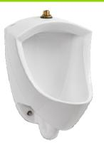
The wall-hung urinal shall be made of vitreous china. Product shall be 22-5/8" in length, 14-5/16" in width, and 14-7/16" in depth. The washdown urinal operates in the 0.125 gpf to 0.50 gpf range. Product has a 3/4" inlet top spud, 2" outlet spud, and includes two wall hangers.
